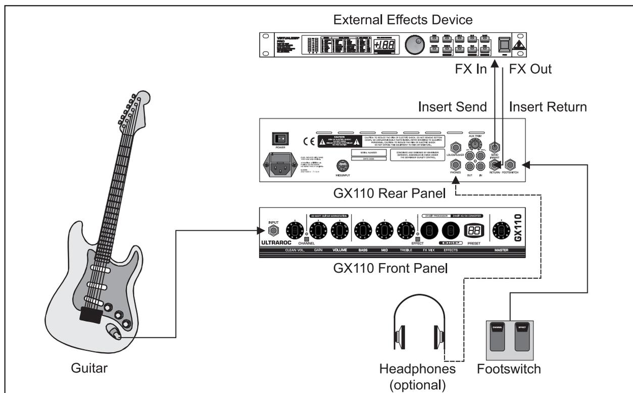
Fig. 2.1: Standard setup
